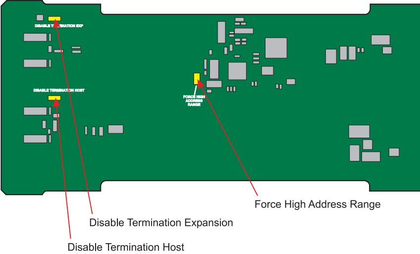
Figure 9 JBOD I/O Module Switch Settings
